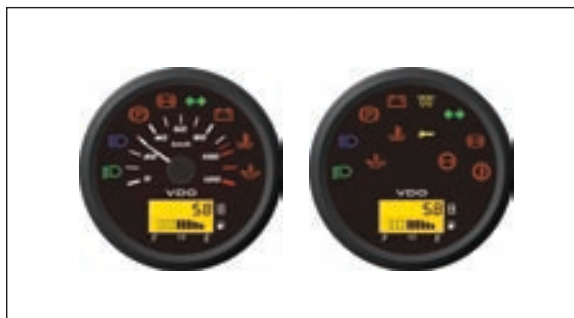
Centrobases instruments with LCD and up to 12 warning lights
